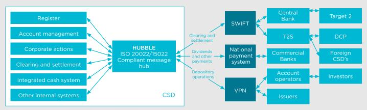
HUBBLE is based on an ESB (Enterprise Service Bus) solution for routing and transforming messages between different information systems. HUBBLE is specifically designed to handle financial market messages defined by ISO standards 20022 and 15022.
